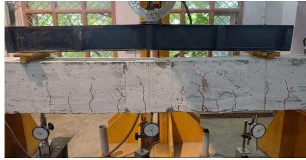
(b) Crack pattern of M40 beam
